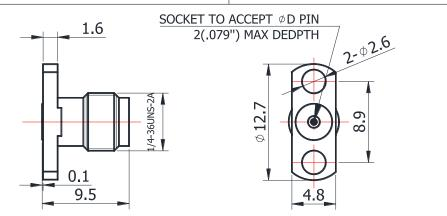
For glass-bead of 0.30mm pin diameter
