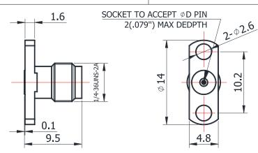
For glass-bead of 0.38mm pin diameter
