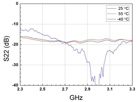
Figure.10 S22 vs Temperature with -12dBm input power
