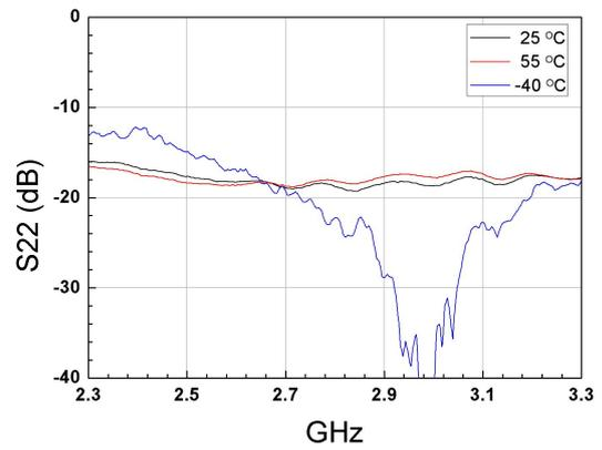
Figure.12 S22 vs Temperature with -10dBm input power
