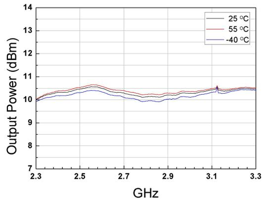
Figure.18 Output Power with -10dBm input power
