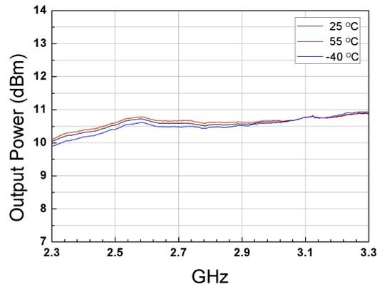
Figure.16 Output Power with -14dBm input power
