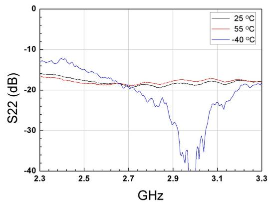
Figure.6 S22 vs Temperature with -16dBm input power
