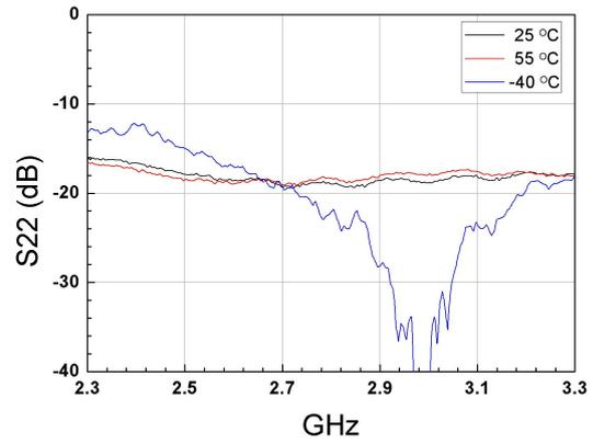
Figure.2 S22 vs Temperature with -20dBm input power
