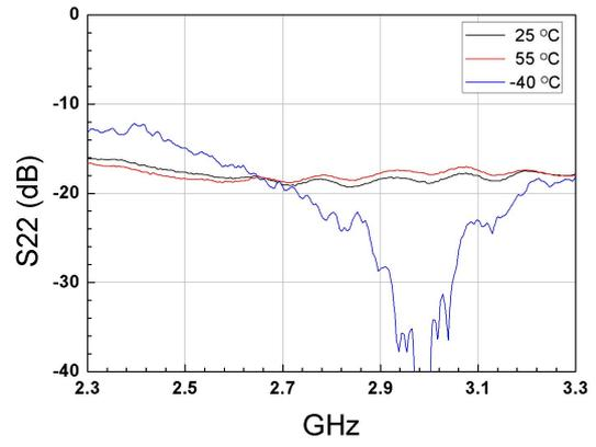
Figure.8 S22 vs Temperature with -14dBm input power
