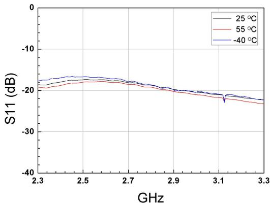
Figure.11 S11 vs Temperature with -10dBm input power
