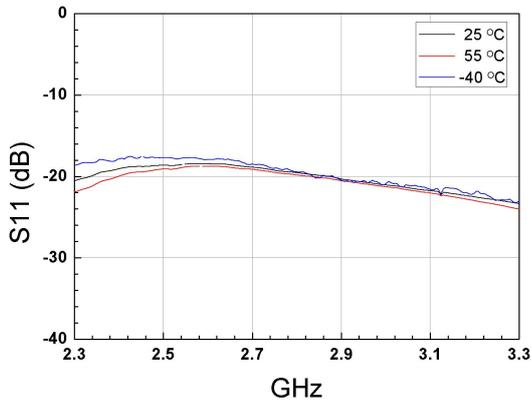
Figure.7 S11 vs Temperature with -14dBm input power
