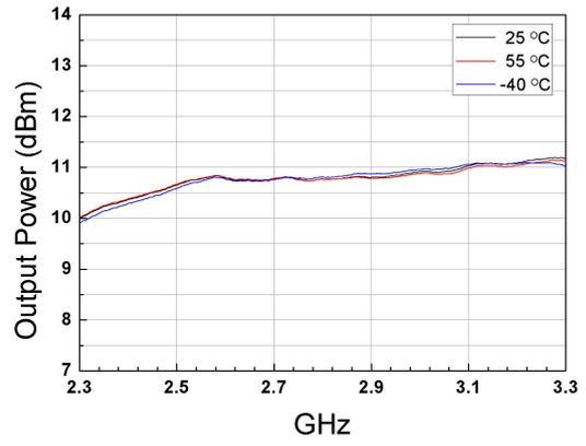
Figure.14 Output Power with -18dBm input power
