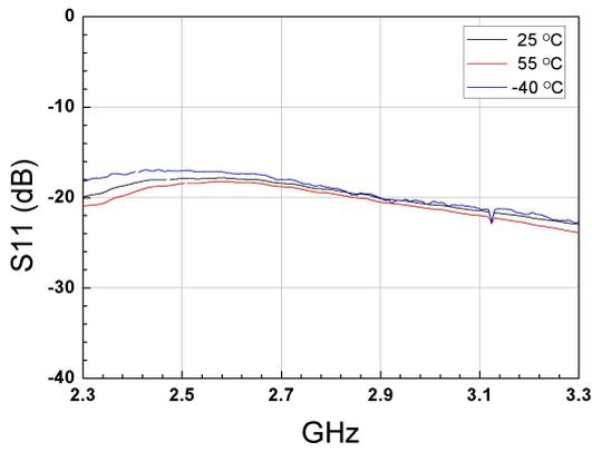
Figure.9 S11 vs Temperature with -12dBm input power
