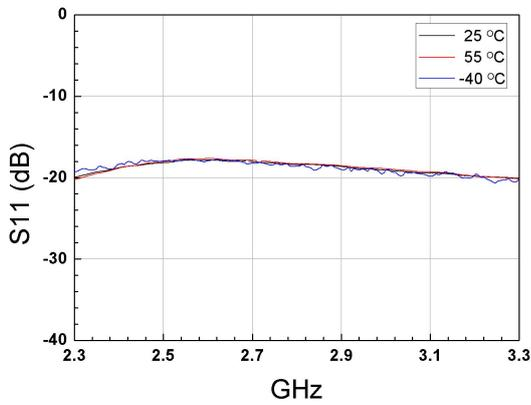
Figure.3 S11 vs Temperature with -18dBm input power
