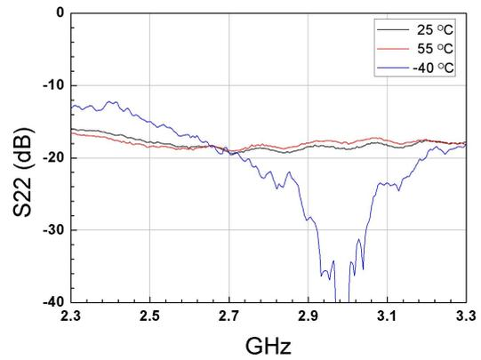
Figure.4 S22 vs Temperature with -18dBm input power
