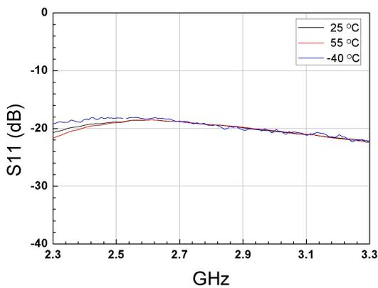
Figure.5 S11 vs Temperature with -16dBm input power
