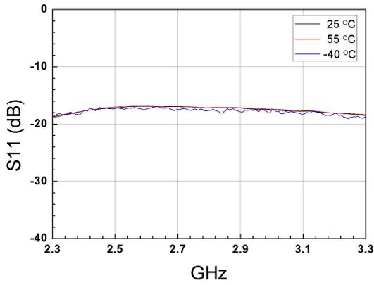
Figure.1 S11 vs Temperature with -20dBm input power
